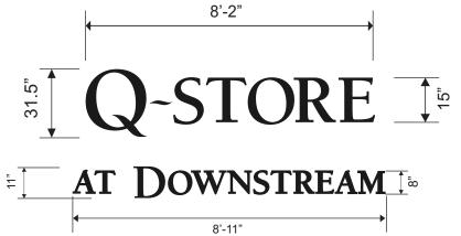
1-SET REVERSE CHANNEL LETTERS WITH LED ILLUMINATED HALO LIGHTING. WIRING RACEWAY ON BACK SIDE
